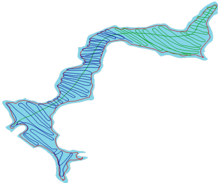
Figure 5.2. Oglethorpe Lake Profile Generated from Sonar Data. Collected sonar data was analyzed via BioBase, a lake monitoring online software. The different colors represent the three different sets of data.
