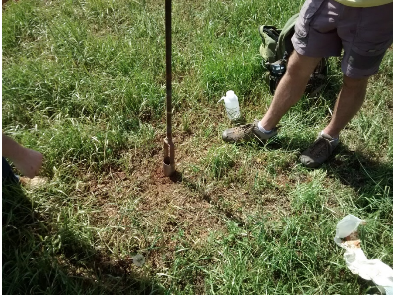
Figure 5.5- Soil sampling technique using steel hand auger in pasture
